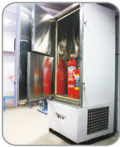
Deep freezer / Internal Corrosion Test
